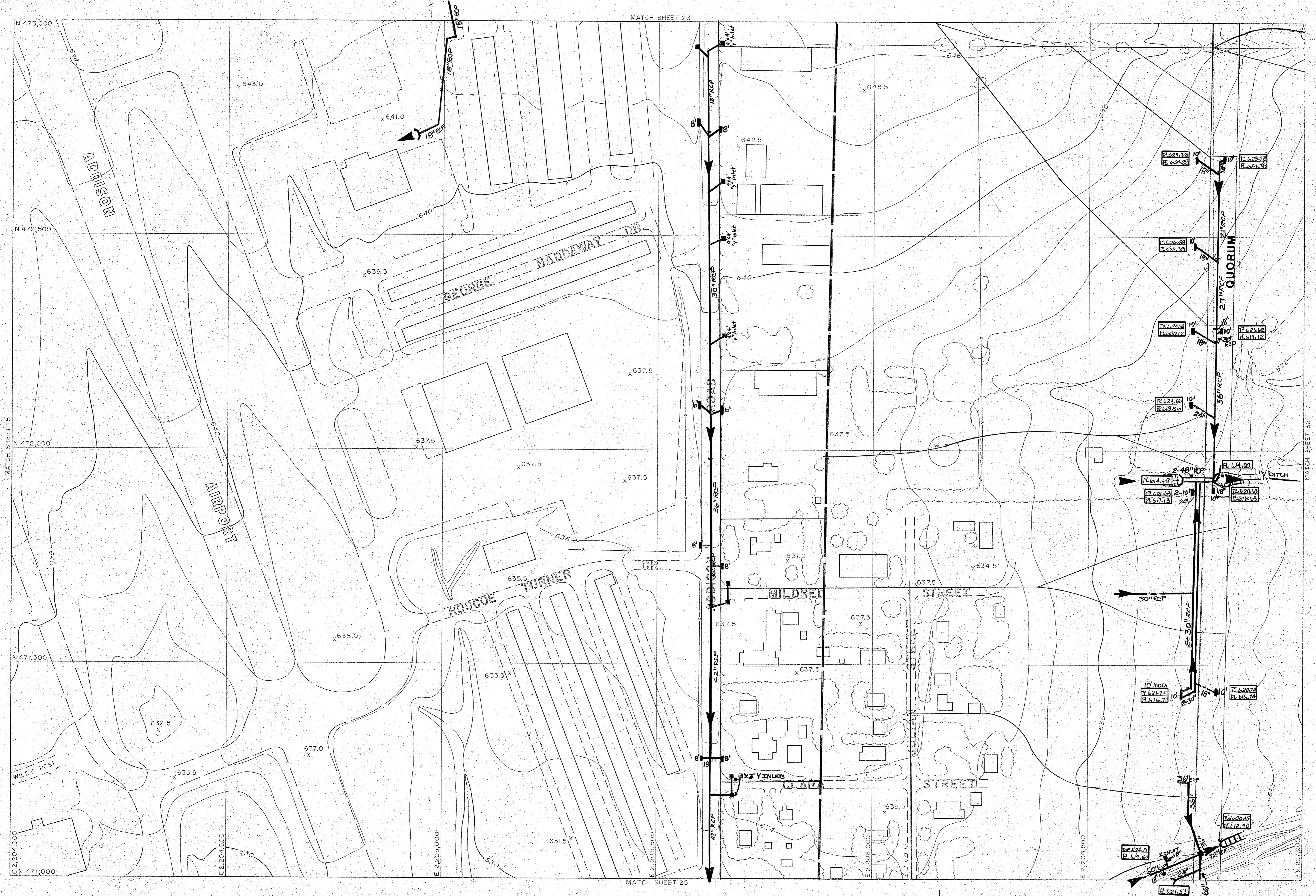
Compiled from aerial photographs taken Nov. 1, 1976 with Wild RC-9 camera. Horizontal Control was extended from existing U.S. Coast and Geodetic Survey monuments by geodimeter and theodolite measurements, with further densification by Aero-Triangular with A-5 Autograph. Vertical control extended from existing U.S.C. and G.S. Bench Marks by spirit levelling.
