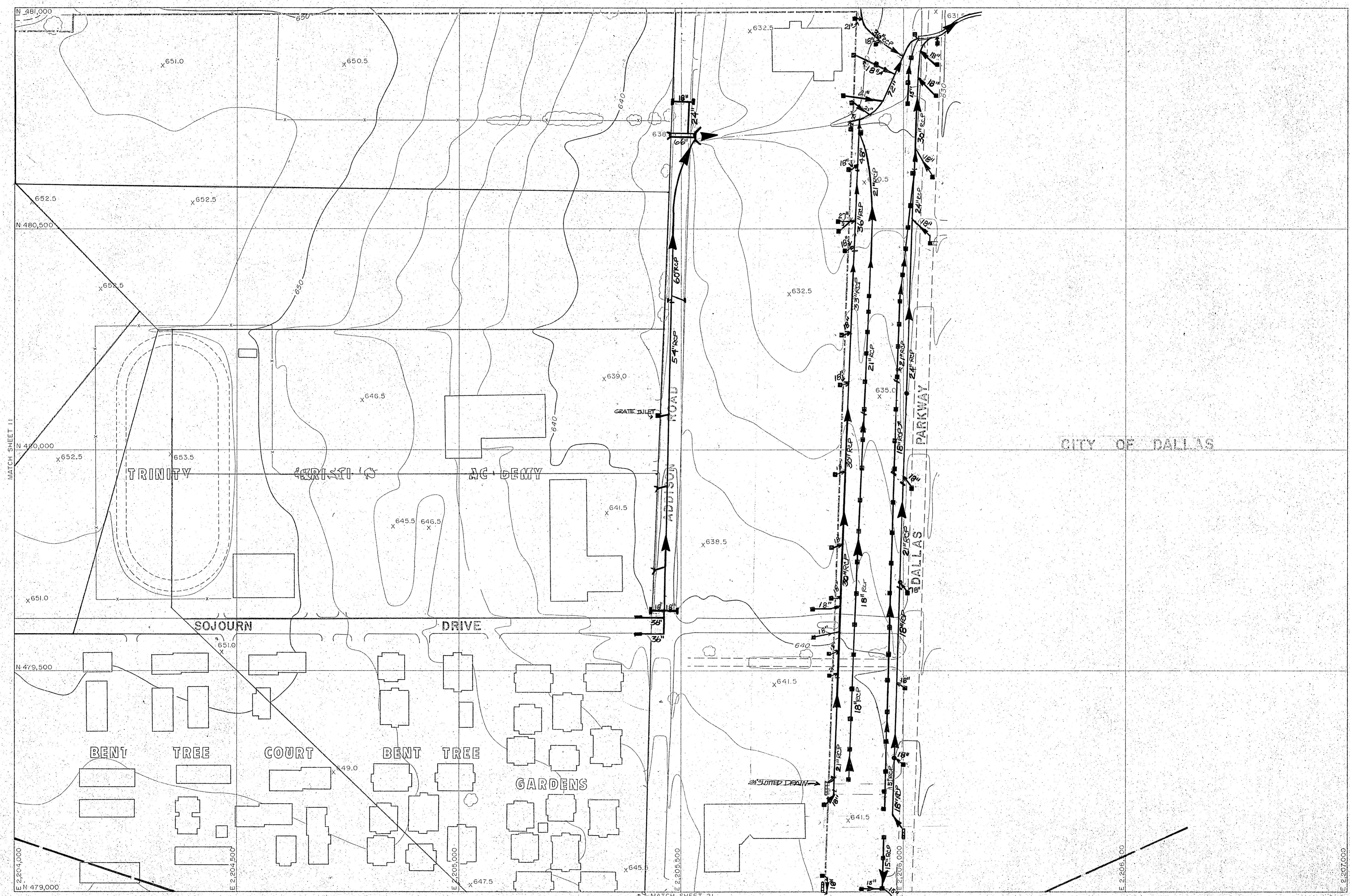
Compiled from aerial photographs taken Nov. 1, 1976 with Wild RC-9 camera. Horizontal Control was extended from existing U.S. Coast and Geodetic Survey monuments by geodimeter and theodolite measurements, with further densification by Aero-Triangular with A-5 Autograph. Vertical control extended from existing U.S.C. and G.S. Bench Marks by spirit leveling.
