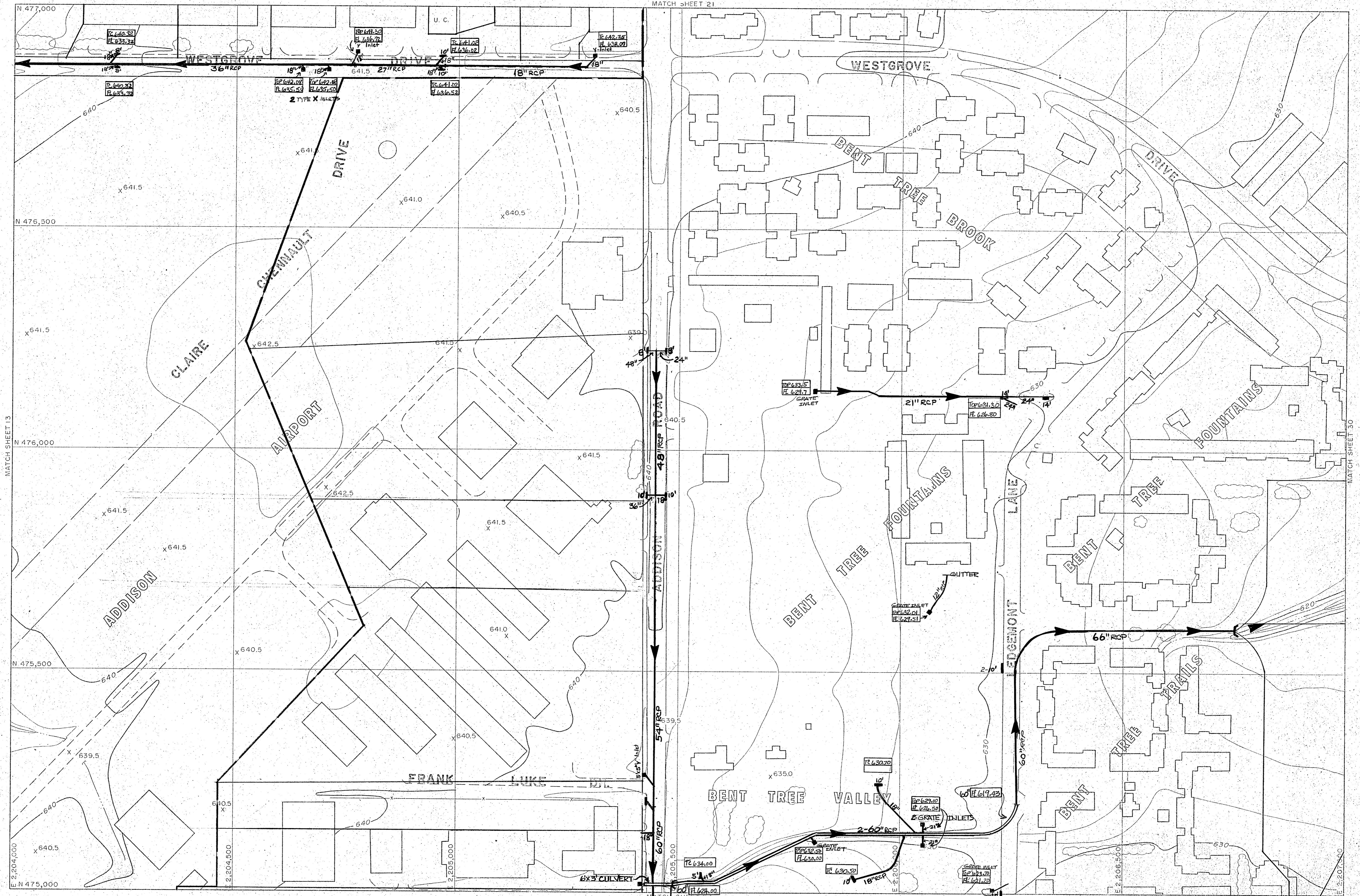
Compiled from aerial photographs taken Nov. 1, 1976 with Wild RC-9 camera. Horizontal Control was extended from existing U.S. Coast and Geodetic Survey monuments by goniometer and theodolite measurements, with further densification by Aero-Triangular with A-5 Autograph. Vertical control extended from existing U.S.C. and G.S. Bench Marks by spirit leveling.
