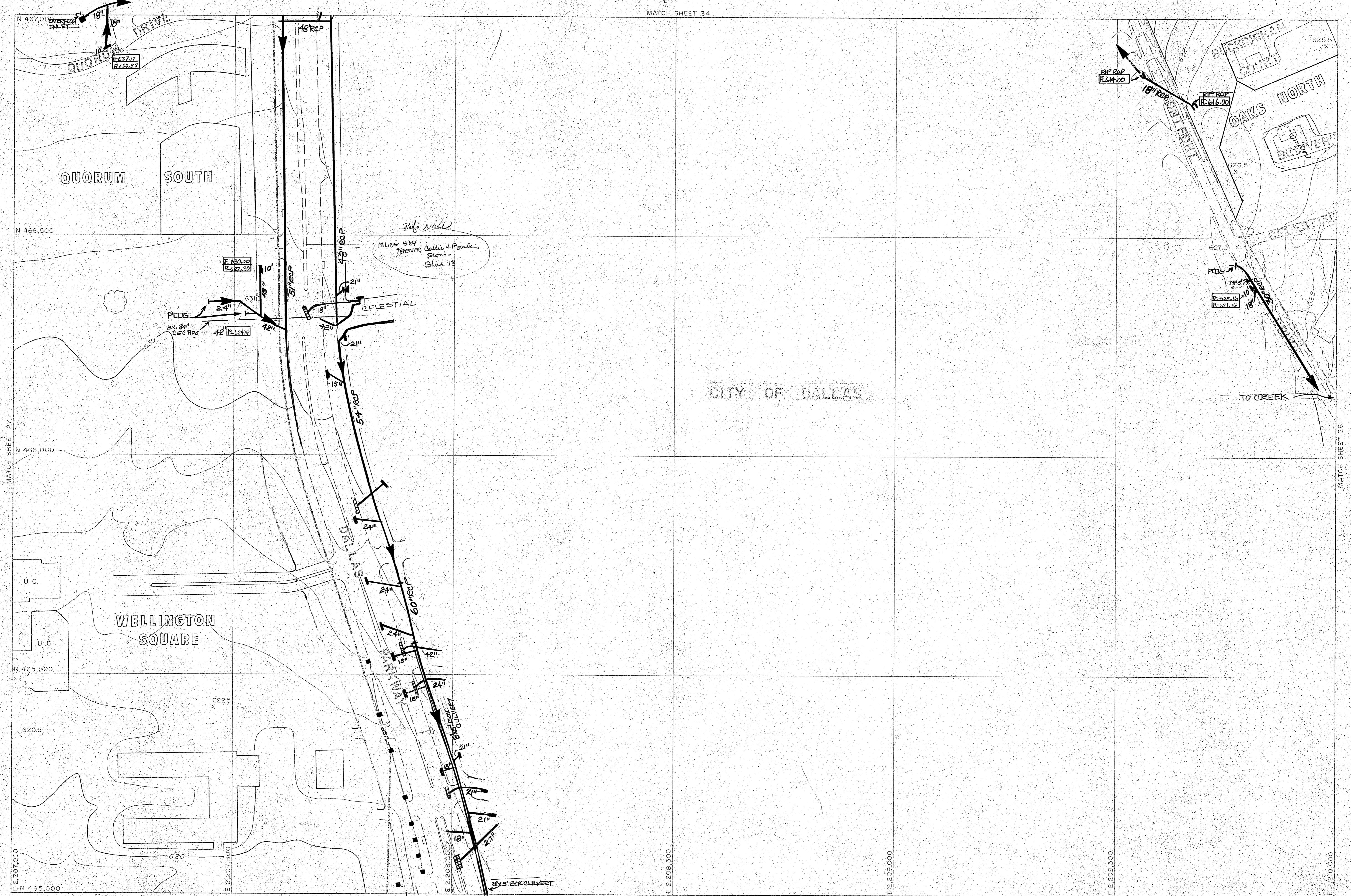
Compiled from aerial photographs taken Nov 1, 1976 with Wild PC-9 camera. Horizontal Control was extended from existing U.S. Coast and Geodetic Survey monuments by geodimeter and theodolite measurements, with further densification by Aero-Triangulation with A-5 Autograph. Vertical control extended from existing U.S.C. and G.S. Bench Marks by spirit leveling.
