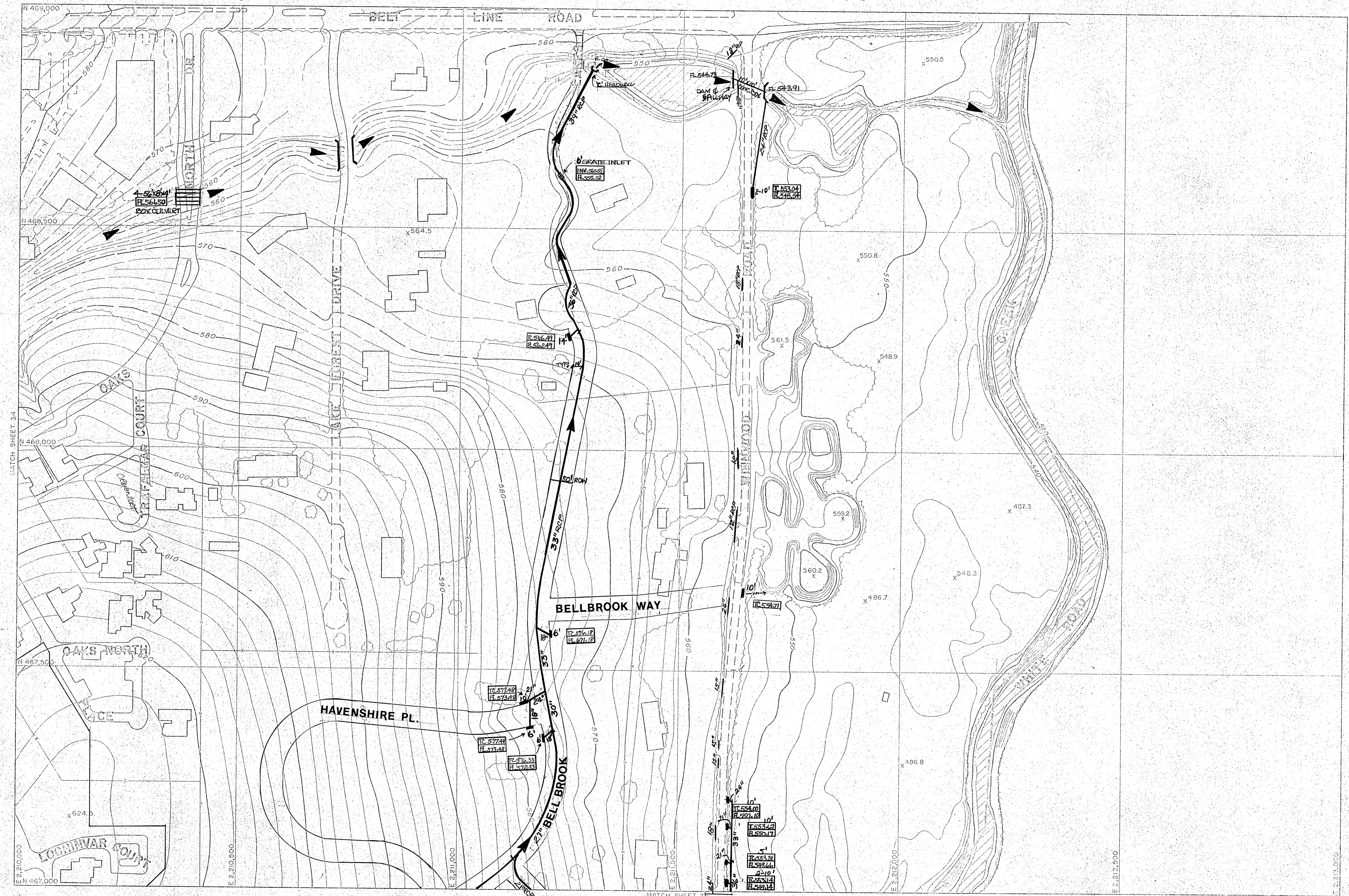
Compiled from aerial photographs taken Nov. 1, 1976 with Wild RG-9 camera. Horizontal Control was extended from existing U.S. Coast and Geodetic Survey monuments by geodimeter and theodolite measurements, with further densification by Aero-Triangular with A-5 Autograph. Vertical control extended from existing U.S.C. and G.S. Bench Marks by spirit leveling.
