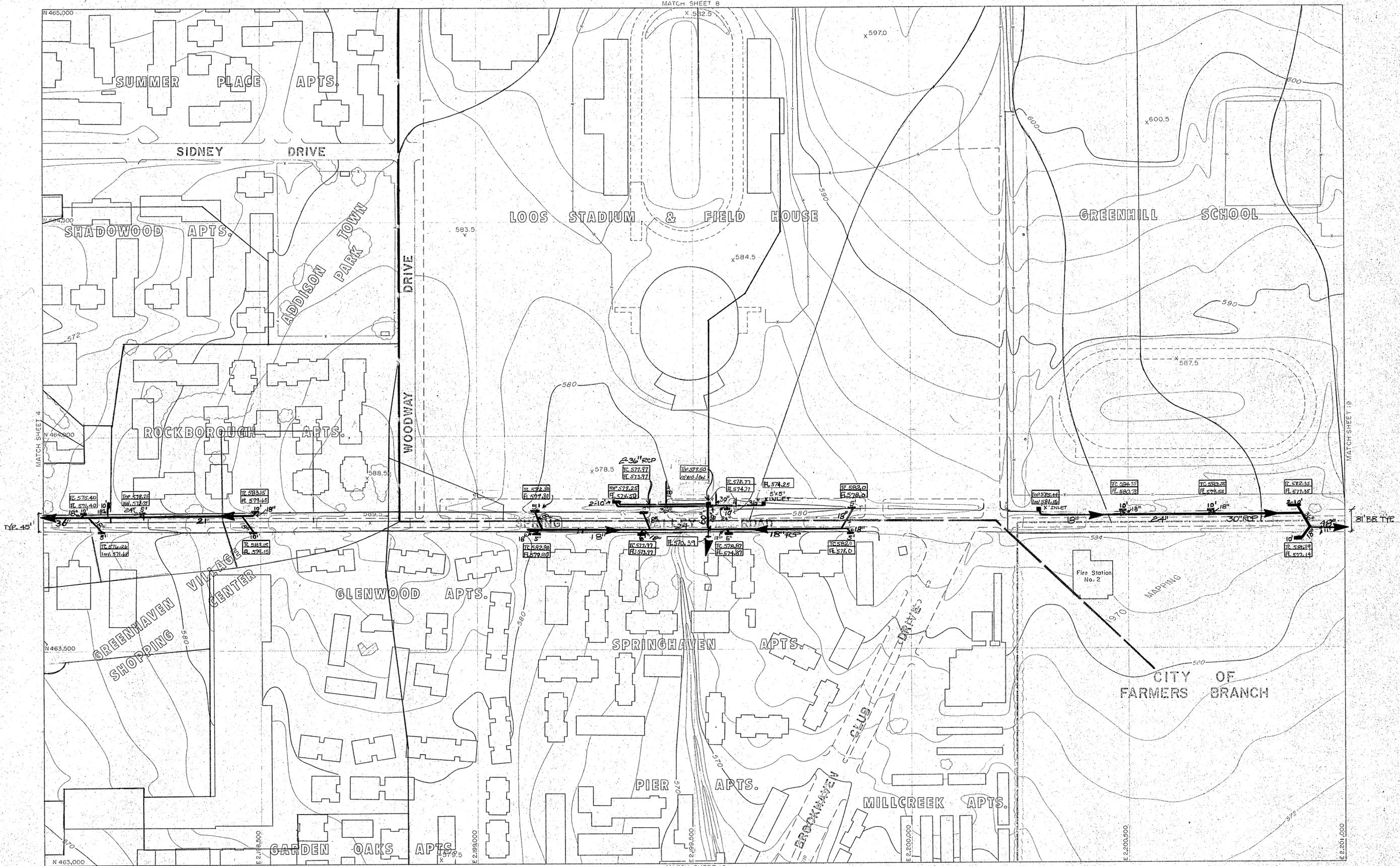
Compiled from aerial photographs taken Nov. 1, 1976 with Wild RC-9 camera. Horizontal Control was extended from existing U.S. Coast and Geodetic Survey monuments by geodimeter and theodolite measurements, with further densification by Aero-Triangular with A-5 Autograph. Vertical control extended from existing U.S.C. and G.S. Bench Marks by spirit leveling.
