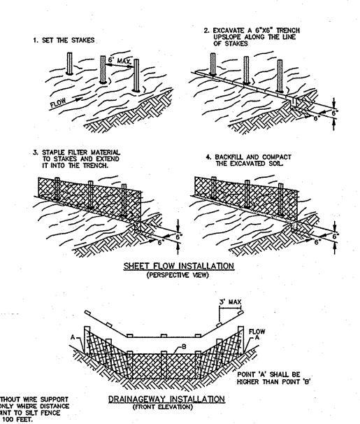
SEDIMENTATION/SILT FENCE WITHOUT WIRE SUPPORT
