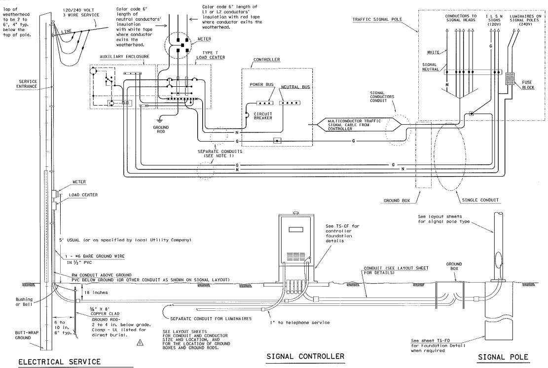
(TYPE T TIMBER POLE SHOWN AS EXAMPLE, SEE ELECTRICAL DETAILS, LAYOUT SHEETS, AND ELECTRICAL SERVICE DATA SHEET FOR SERVICE REQUIRED AND FOR DETAILS.)
