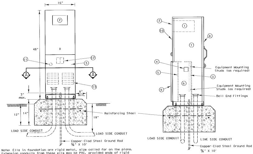
Extension conduits from these ells may be PVC, provided ends of rigid metal conduits are more than 2 in. below top of concrete foundation. Where extension conduits are metal, grounding bushing must be installed and a bonding jumper properly terminated.
