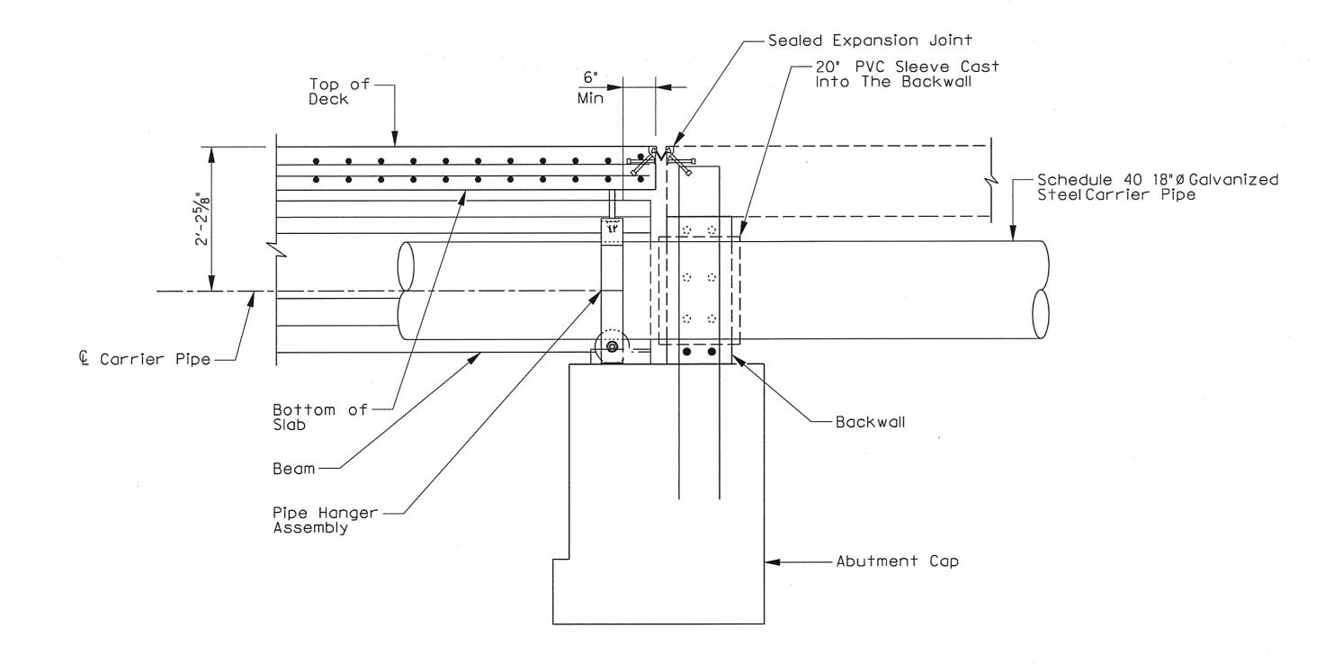
PIPE HANGER ASSEMBLY TYPICAL SECTION
