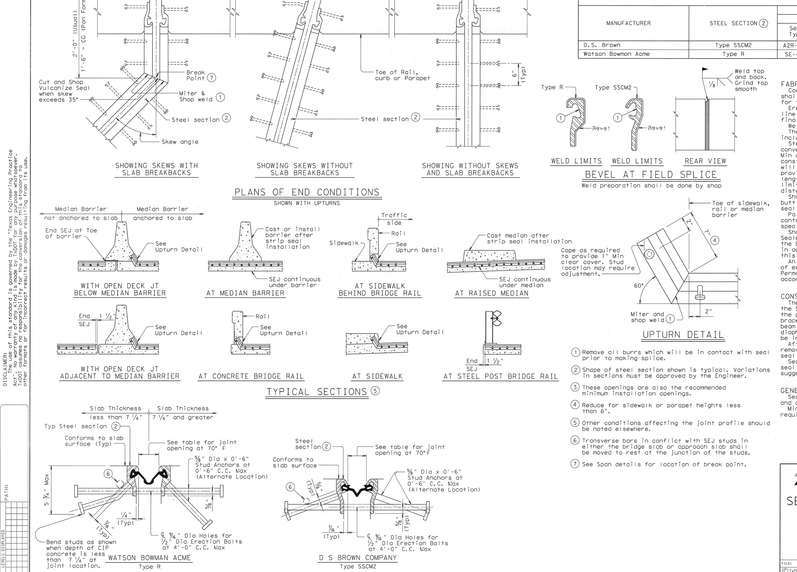
SECTIONS THRU SEALED EXPANSION JOINT
