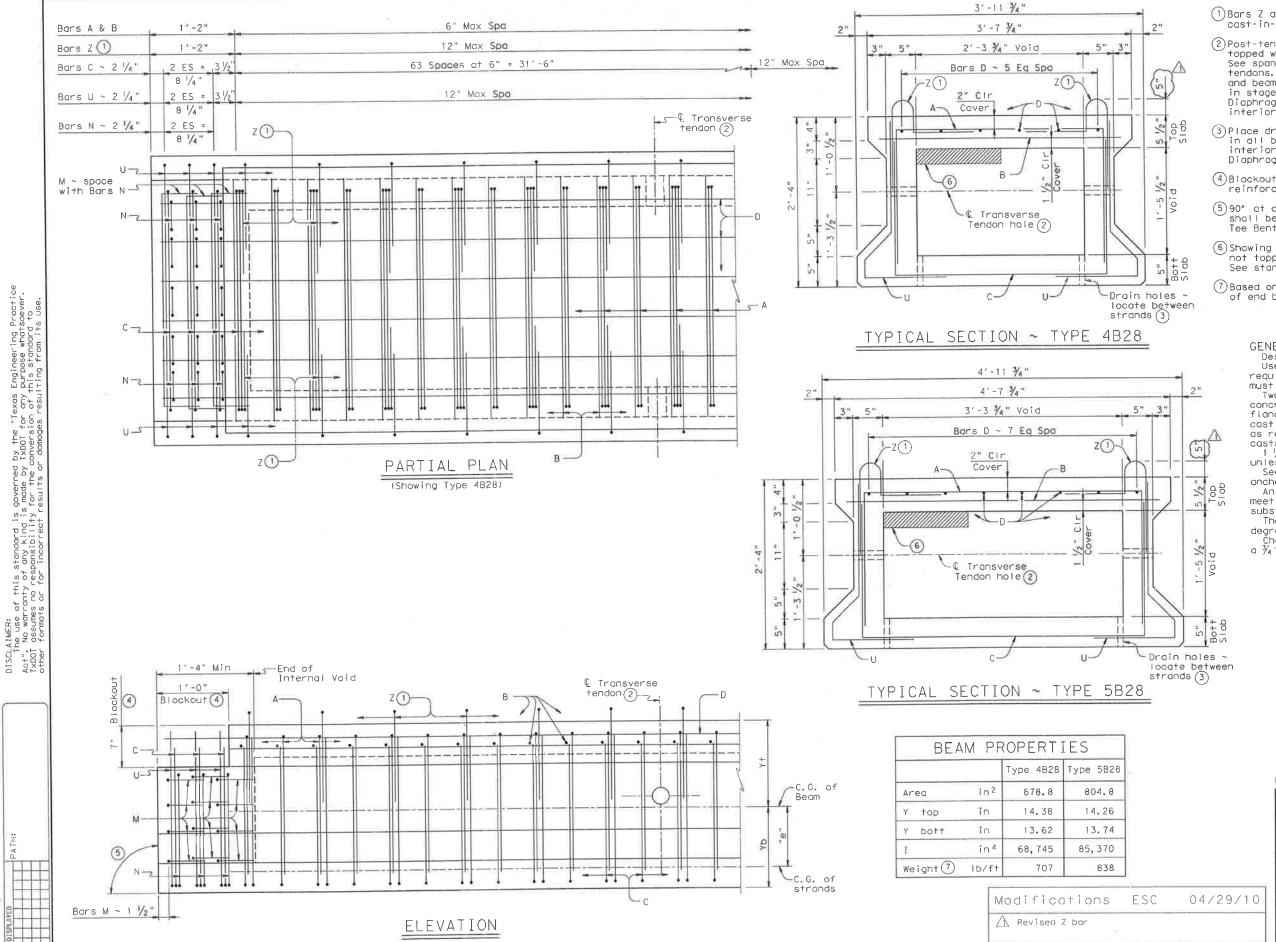
(1) Bars Z are required for beams topped with a cast-in-place concrete slab only.
