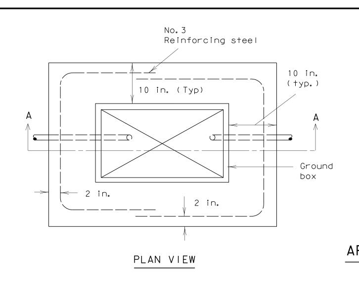
(1) Final position of end of conduit shall not exceed one-half the distance to the side of box opposite the conduit entry. (2) Place gravel "under" the box. not "in" the box. Gravel should not encroach on the interior volume of the box.
