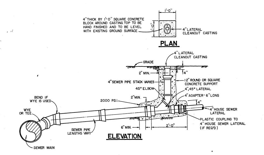
ALL PVC SANITARY SEWER PIPE TO BE SDR 35 WITH INTEGRAL BELL.
