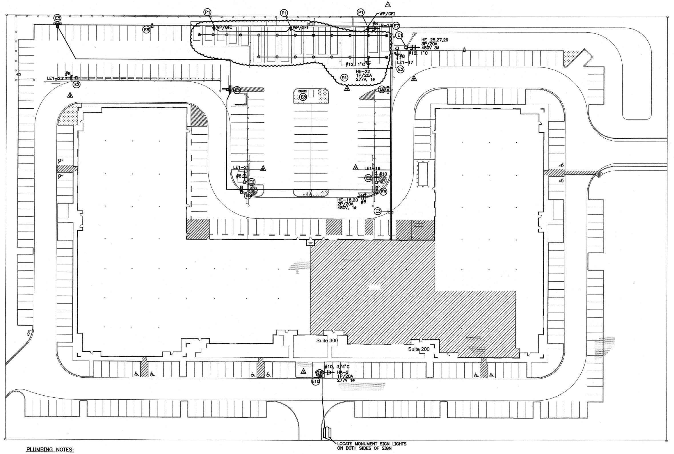
P1 PROVIDE YARD HYDRANT EQUAL TO WOODFORD MODEL S3, BACKFLOW PROTECTED, AUTOMATIC DRAINING AND FREEZELESS.
