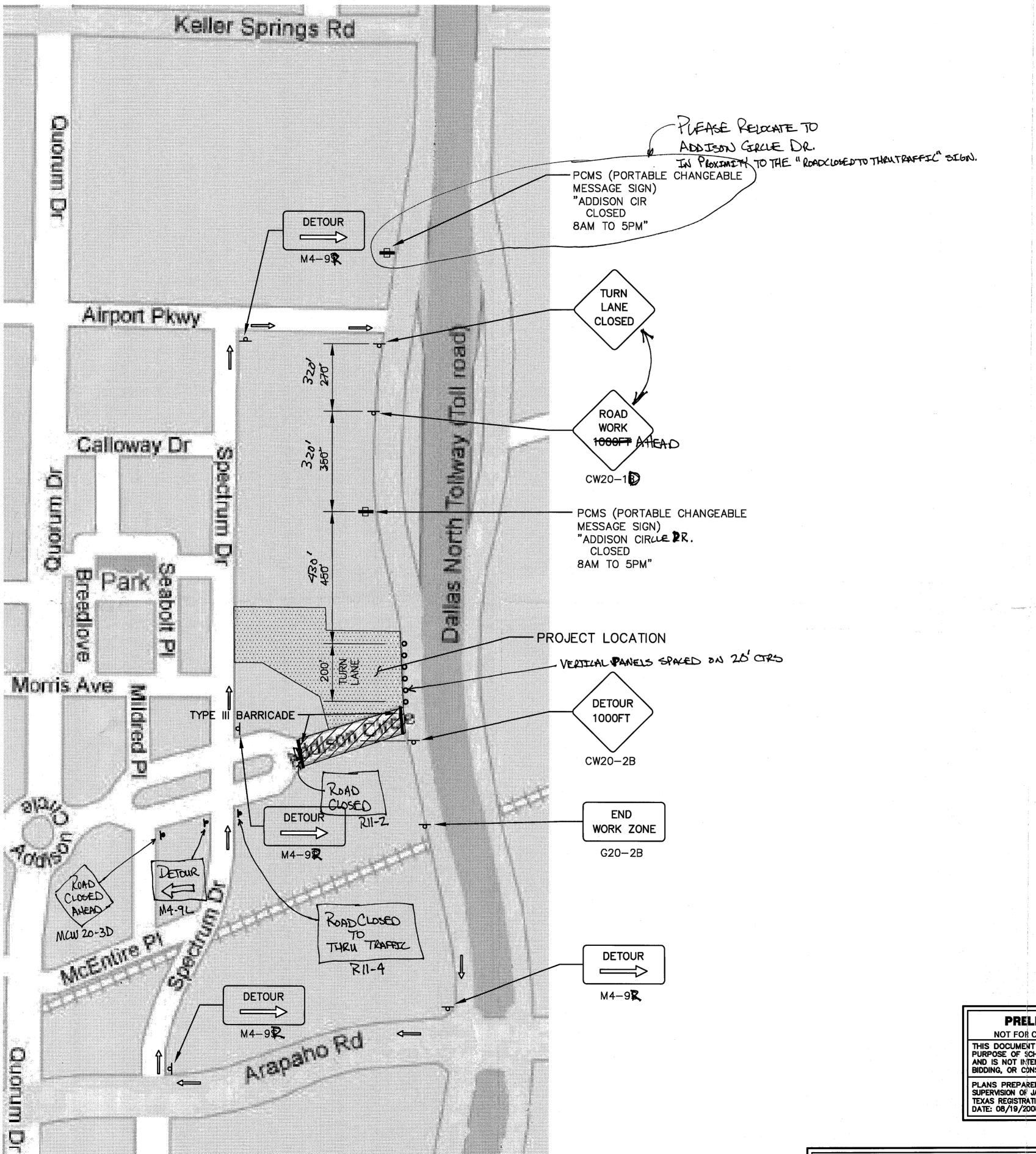
PCMS (PORTABLE CHANGEABLE MESSAGE SIGN) "RIGHT LANE CLOSED 8AM TO 5PM" ROAD CLOSURE
