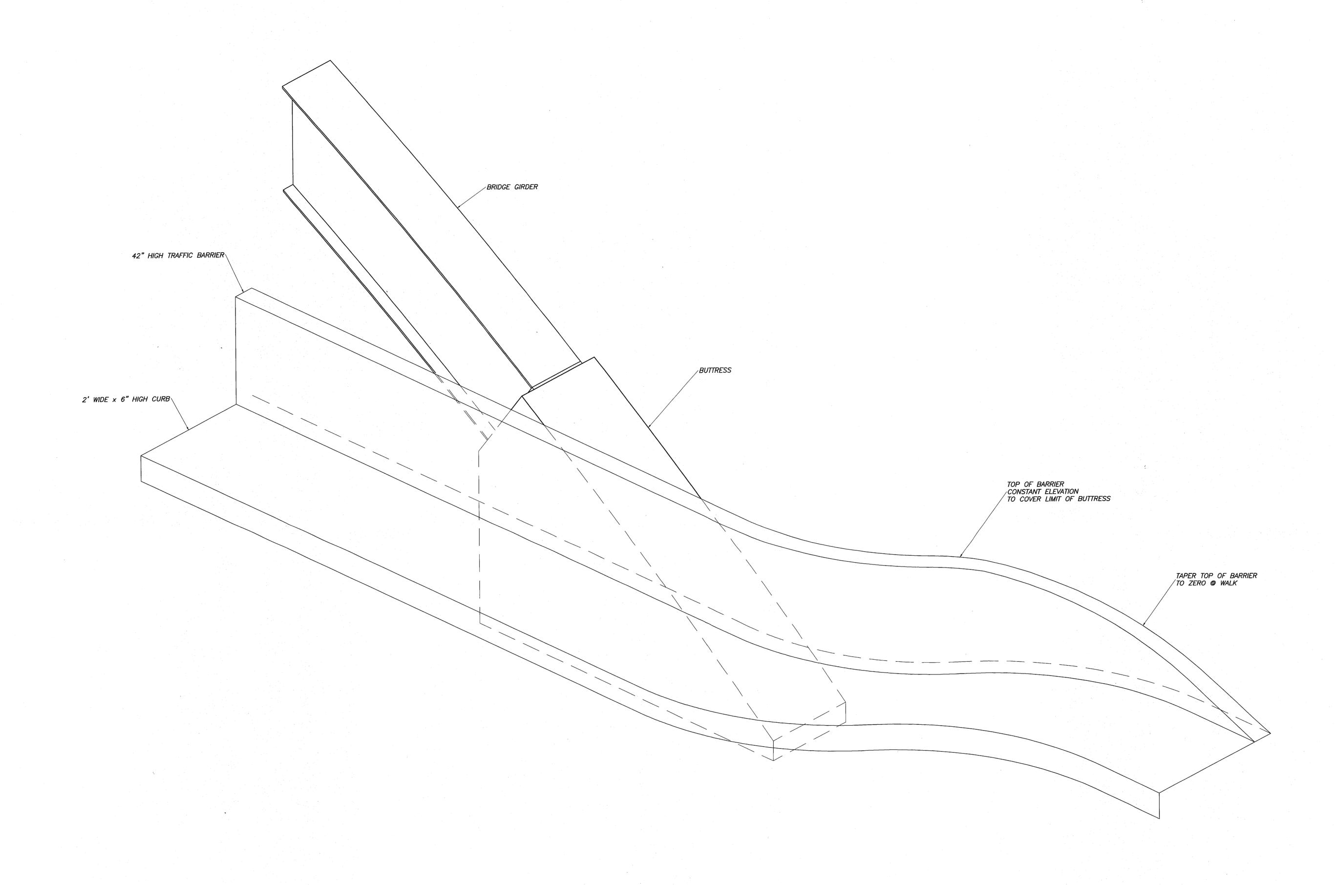
ISOMETRIC VIEW OF BUTTRESS END TREATMENT
