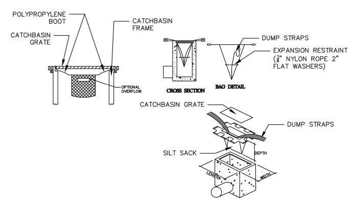
THIS METHOD OF INLET PROTECTION IS APPLICABLE WHERE THE INLET DRAINS SHEET, OVERLAND AND CONCENTRATED FLOWS (NOT GREATER THAN 1 CFS). THE METHOD CAN DRAIN FLAT AREA TO STEEP SLOPES. INLET CAPACITY WILL DECREASE WITH THIS METHOD AND CONTRACTOR SHALL EXPECT FLOODING TO OCCUR DURING HIGH FLOW EVENTS.
