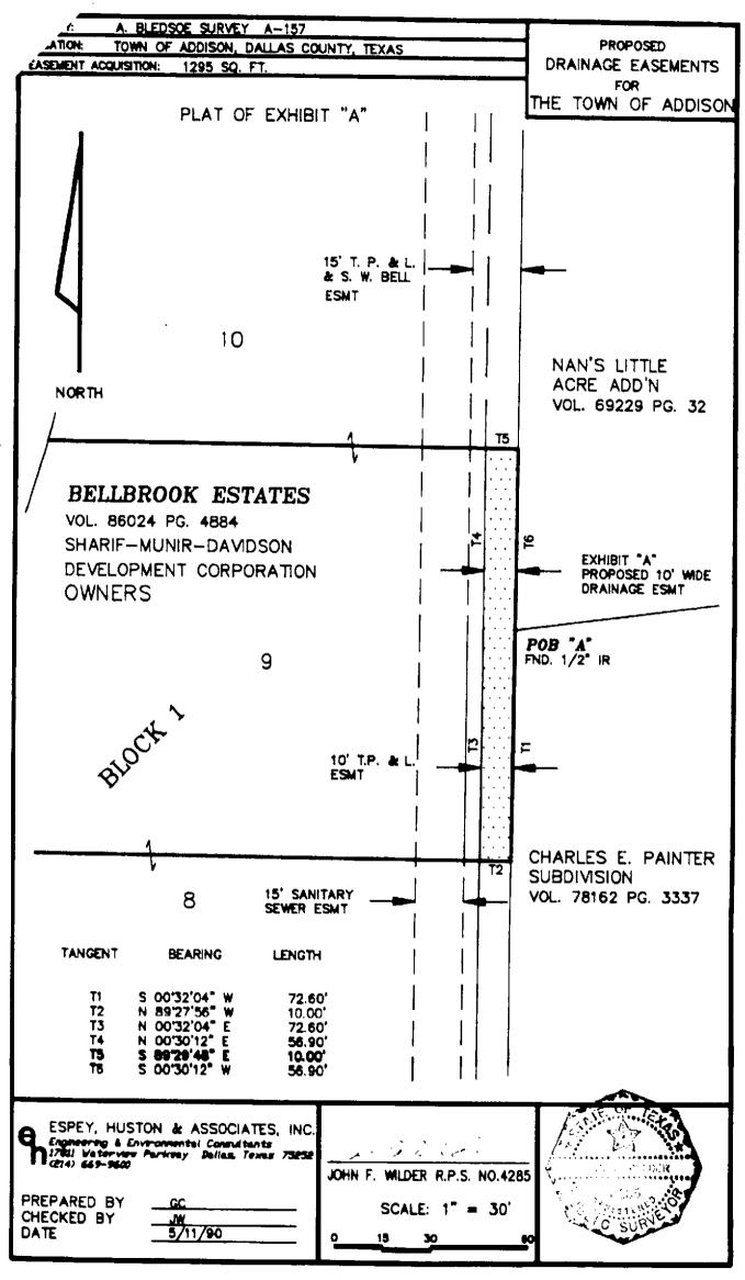
A 10-FOOT WIDE STRIP OF LAND FOR A DRAINAGE EASEMENT, BEING A PART OF LOT 8, BLOCK 1, BELLBROOK ESTATES, AS RECORDED IN VOLUME 86024, PAGE 4884, OF THE PLAT RECORDS OF DALLAS COUNTY, TEXAS (PRDCT), BEING OUT OF THE A. BLEDSOE SURVEY, ABSTRACT NO. 157, IN THE TOWN OF ADDISON, DALLAS COUNTY, TEXAS, AND BEING MORE PARTICULARLY DESCRIBED AS FOLLOWS:
