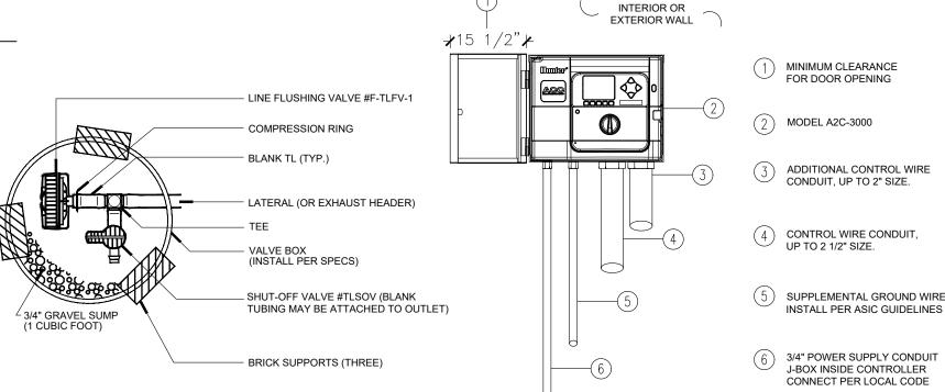
LINE FLUSHING VALVE **HUNTER ACC CONTROLLER - WALL MOUNT** W/ SHUT-OFF VALVE
