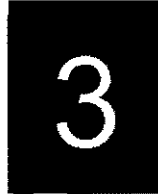
Runway Distance Remaining Signs
