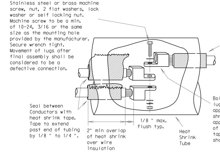
Increase insulation diameter with heat shrink tape if necessary. Tape to extend past end of tubing by 1/8 " to 1/4 ".
